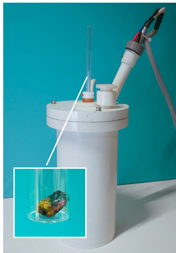
Fig. 6 SPAQ device with a SLN situated in the glass sample holder
