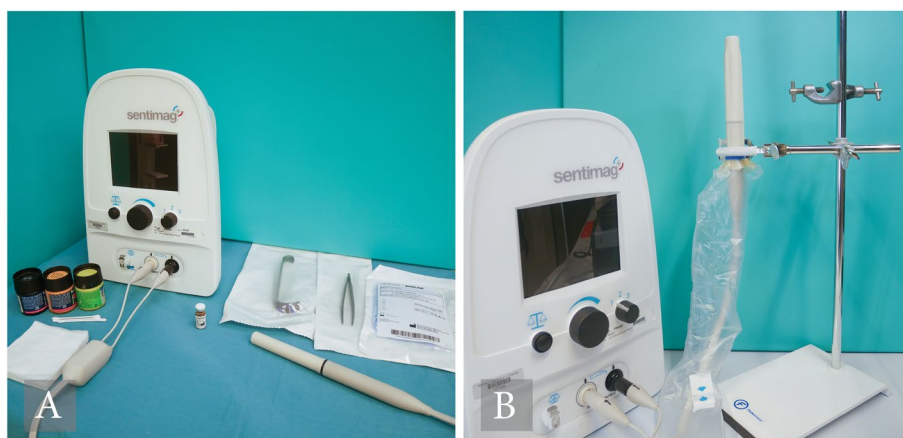
Fig. 4 Sentimag setup during surgery ( A ) and ex-vivo measurements ( B )
